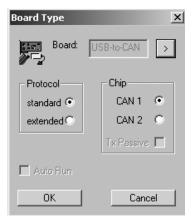
Confirm your input. The USB interface will now be tested. If the transfer test was successful it will be indicated in the CAN Status window.
